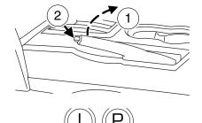
**WARNING:** Always set the parking brake fully and make sure that the gearshift is securely latched in P (Park) (automatic transmission) or in 1 (First) (manual transmission).
